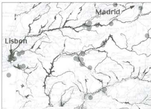
Fig. 1. In the May 20, 2003 dx opening, sixty percent of the radio paths between the Canary Isles and central Europe show midpoints which appear to correlate to the position of lakes and major rivers in Spain and Portugal [2].
